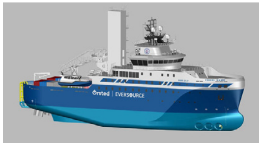
Offshore wind Service Operations Vessel (SOV) design [Image: Ørsted]
